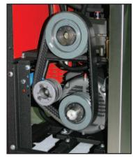
Vertical banded belt provides extended life and reduced maintenance costs by eliminating multiple belts that stretch at different rates. New belt tensioner provides constant tension and makes servicing and maintenance of the belt a breeze.
