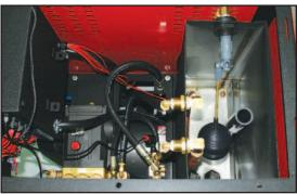
Large 10-gallon polyethylene float tank with cool-down pump by-pass loop to significantly reduce potential pump damage from the operator regularly running the machine in by-pass mode.
